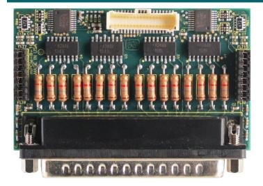
The Isolation Module includes jumpers to enable input filters with a 4.7ms time-constant, optimized for dealing with AC signals, but useful for a wide variety of transient-mitigation tasks.
